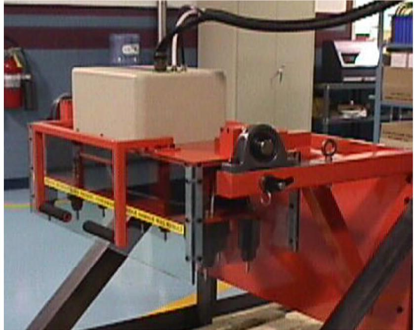
**The TMM7200 Marking Head/Manifold Assembly in the downward facing, marking orientation.**
