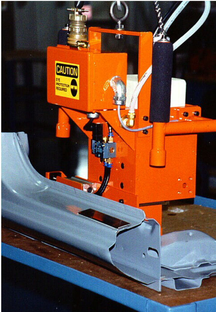
TMM5100 Marking Head with custom pneumatic clamp holds the marker in place during the print cycle.
